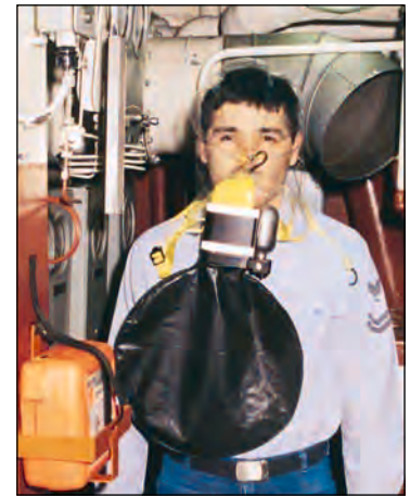
The Ocenco M-20.2 EEBD shown donned and ready for escape.
